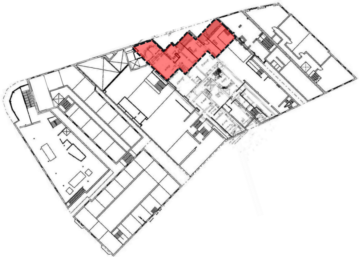
Figure 4 5a: Ground level plan of the Bourbon showing the extent of existing facade and internal fabric to floors and walls to be retained in dotted black outline, shaded in red
