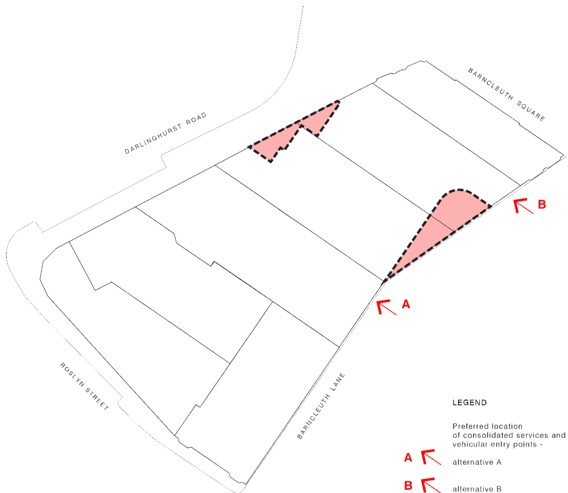
Figure 9: Plan of the development block showing areas within the site to be redesigned as extensions and enhancements to the adjacent public domain (shaded in red/black dotted line)
